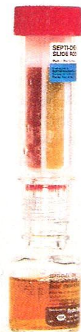
Figure 52-5 Becton Dickinson Septi-Chek pediatric-size biphasic blood culture bottle. The medium-containing base bottle is inoculated with blood, and the top piece containing agar paddles is added in the laboratory. The agar is inoculated by tipping the bottle to allow the blood-containing medium to flow over the agar.
